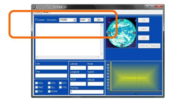
5. Click **On** button to establish the communication between BT-Q1300ST and your PC. If the connection is successful, the NMEA stream will keep showing.
