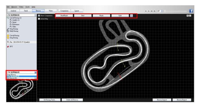
There is only one beacon type for drag racing; all you have to do is to use "Set Valid lap" beacon type to mark the valid laps of your track. QRacing will automatically calculate and analyze for this racing type by user-defined distance or speed.
