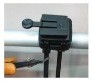
5. Upon completion, slide in Q2100 along the direction indicated by the arrow in the figure until it snaps.
