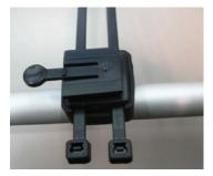
3. Fasten the cable ties around the horizontal bar of the bicycle.
