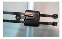
3. Fasten the cable ties around the vertical bar of the bicycle.
