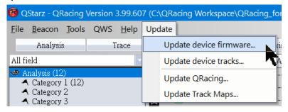
QRacing will check and update to the latest software version when there is a new version released. If your Qstarz device is connected to QRacing, it will also check the firmware version. For firmware update, please visit Racing.Qstarz.com for more information.
